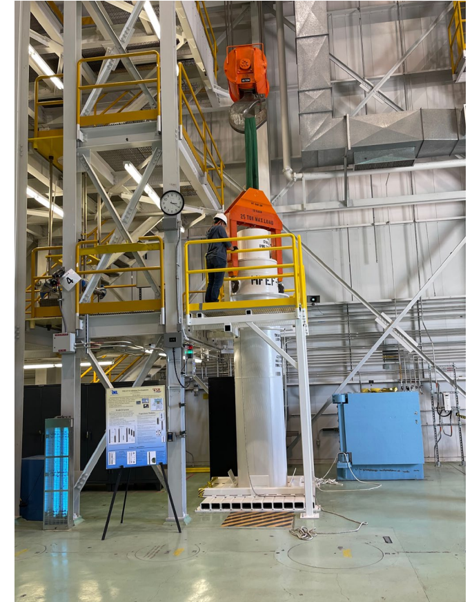
HFEF-15 Cask in cask stand at TREAT awaiting transient testing
