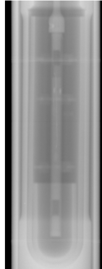
Left: neutron radiography post transient showing intact rodlet. Above: post transient dimensional inspection showing diametral strain and no axial strain.
